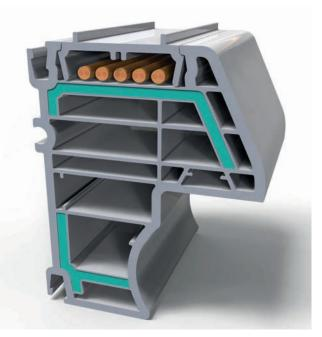
**Fig. 4.** Door profile of a chest freezer: hereby, Ultradur replaces a metal stiffener, which eliminates the need for an electrical heater in the profile to prevent condensate formation on the outer surface. This improves the freezer's energy efficiency.
