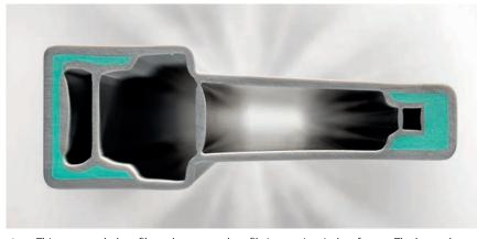
Fig. 2. This co-extruded profile replaces a steel profile in certain window frames. The lower thermal conductance increases the energy efficiency. © Profine
