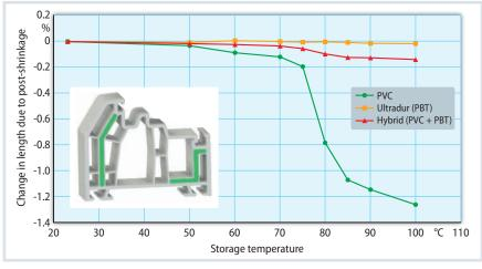
**Fig. 1.** Permanent post-shrinkage of profiles made of rigid PVC and the PBT Ultradur from BASF, as well as hybrid profiles of PVC and PBT after heating to a certain temperature: shrinkage of hybrid profiles is significantly lower than with pure PVC profiles. On average, the measured hybrid profiles contain about 18 % PBT. Source: BASF; graphic: © Hanser
