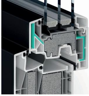
Fig. 3. Ultradur B4040 G11 HMG HP can be used instead of steel to stiffen rigid PVC profiles. The result is a lower permanent deflection after one-sided heating. Moreover, thermal conductance is reduced. This permits large, energy-saving windows, also with dark-colored profiles.
